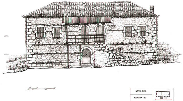
Fig. 9. Academic Year 2009-10. Traditional houses in the Municipality of Trikala, Prefecture of Korinth. Elevation showing defects.
