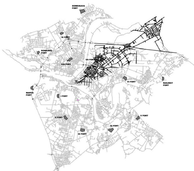
Fig. 1. Global depth map of Kaunas and locations of Forts (black colour indicates five percent of the shallowest axes). Map by Kęstutis Zaleckis and Giedre Gudzinevičiūtė
